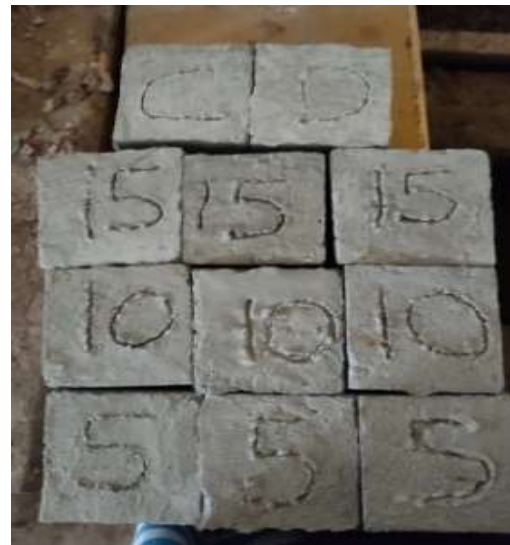
Fig. 3. The cube specimens after 7- and 28-days curing.
