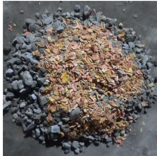
Fig. 2. Crushed waste plastic mixed with cement, fine aggregate and coarse aggregate
