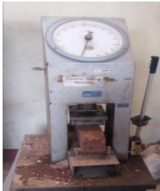
Fig. 3: Specimen placed on Flexural testing machine
