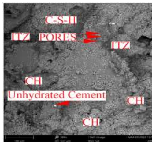
Fig 13. Scanning electron microscopy of concrete specimen used for rapid chloride penetration test at day 28.
