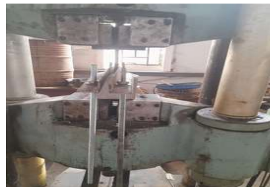
Fig. 4: Rebar pulled out from cube
