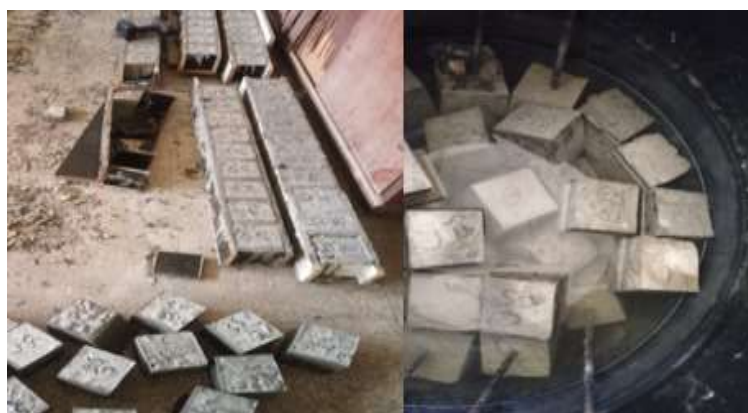
Fig. 1: Removal of formwork and curing of cubes in salt water
