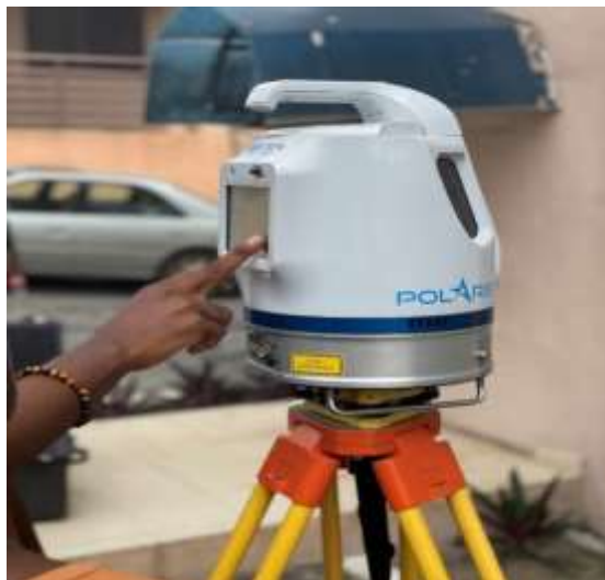
Fig 4: The setup of a LASER scanner during a scanning operation
