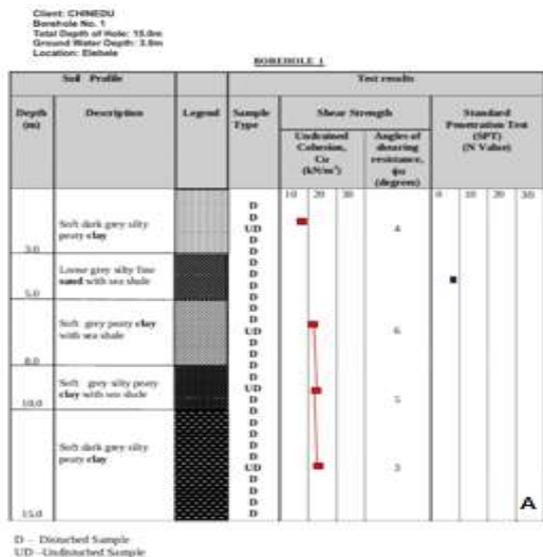
Fig. 2 (A). Borehole log for BH1
