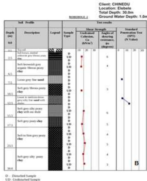
Fig 2 B Borehole log for BH2
