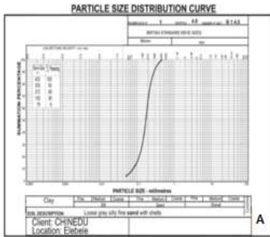
Fig.3 Particle size distribution curve BH1 @ 4.0m
