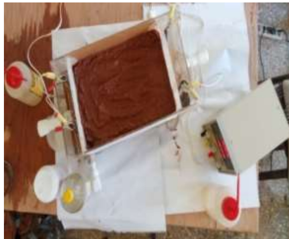
Fig. 1: Cosolvents Enhanced Electrokinetic Remediation Set-up
