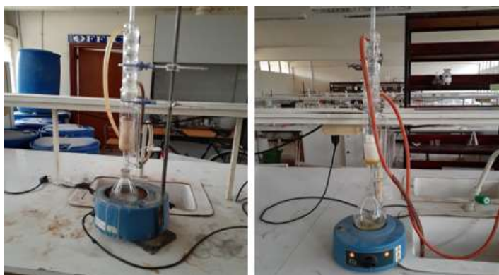
Fig 2. Soxhlet extraction of oils from Trichilia dregeana seed beans and their shells (Photo: Phillip T., April, 2021).
