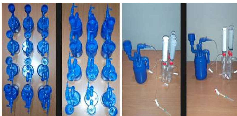
Fig 1. 2L-Capacity anaerobic digester with biogas cleaning system and gas measuring
