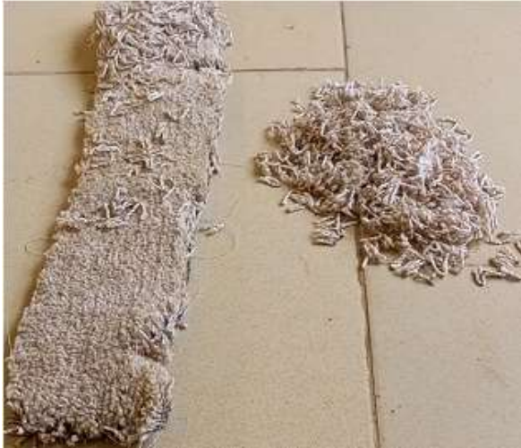
Plate 1 Removal of the Yarn from the Carpet
