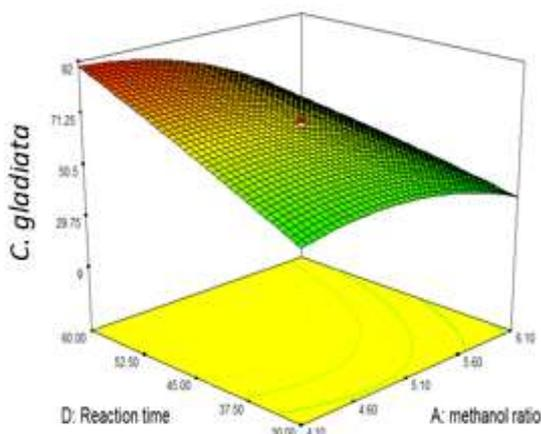
Fig 2: Response Surface Plot showing the Effect of Reaction Time and Mole ratio on Biodiesel Conversion
