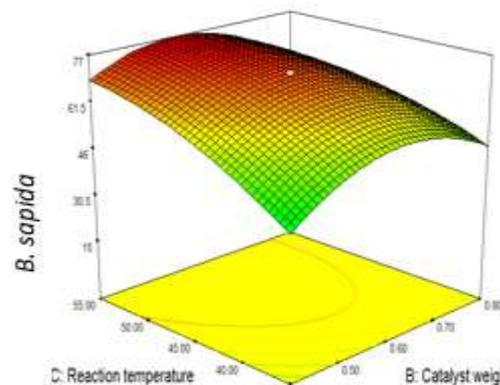
Fig 5: Response Surface Plot showing the Effect of Reaction Temperature and Catalyst concentration on Biodiesel Conversion
