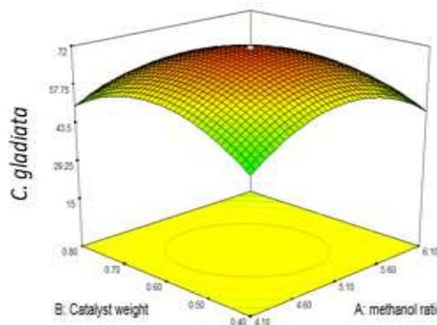
Fig 3: Response Surface Plot showing the Effect of catalyst concentration and mole ratio on Biodiesel Conversion
