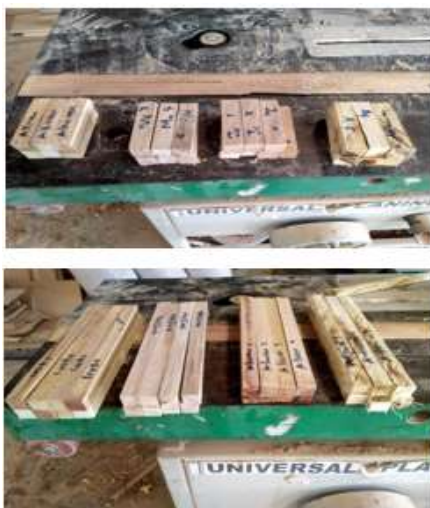
Plate 1: Samples for determination of basic physical and mechanical properties
