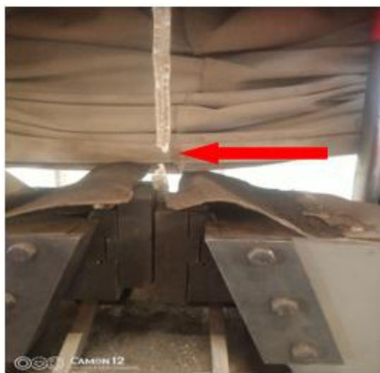
Fig 2: Image of Sample after Elongation Showing Breakage
