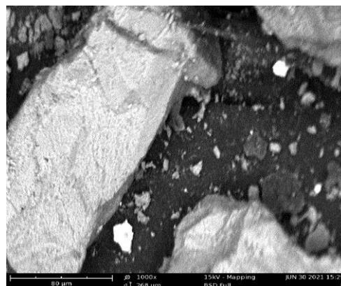
Fig. 5: SEM micrograph of modified groundnut shell
