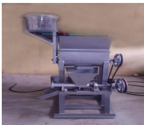
Fig 3. Pictorial View of the completed mixing and pelletizing machine
