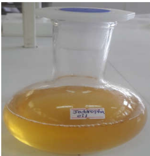
Figure 3. The oil extracted from Jatropha curcas seeds using soxhlet extractor
