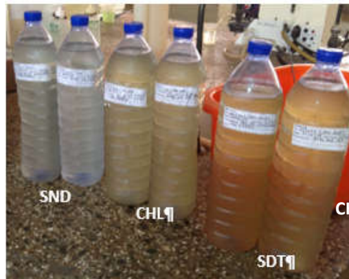
Fig 3: Effluents from Sand (SND), Charcoal (CHL) and Saw dust (SDT)
