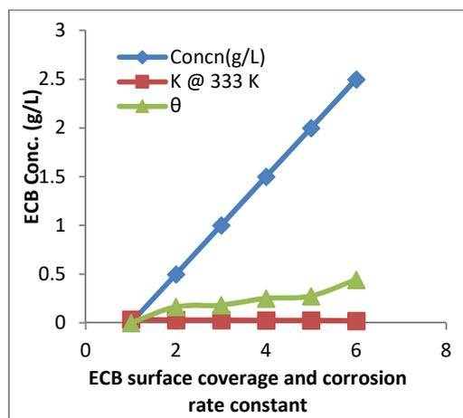
Fig.8: ECB concentration against ECB surface coverage and corrosion rate constant for pipeline steel corrosion in acidic environment at 60 °C (333 K)
