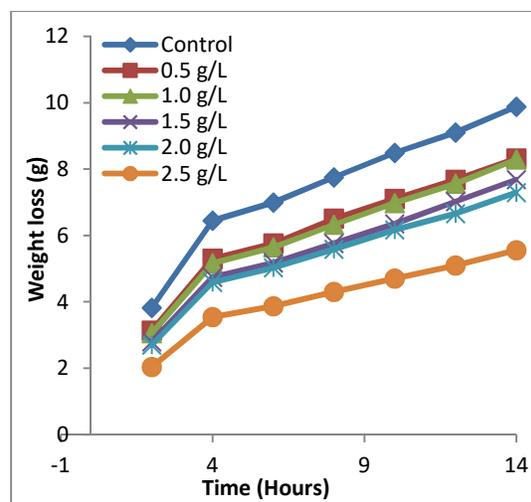
Fig.3: Variations in weight loss with time for pipeline steel coupons in 0.5 M H<sub>2</sub>SO<sub>4</sub> solution containing different concentrations of *Enantia chlorantha* at 60 °C
