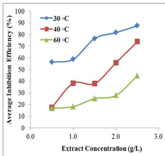
Fig.4: Variations in average inhibition efficiency at different ECB extract in 0.5 M H<sub>2</sub>SO<sub>4</sub>
