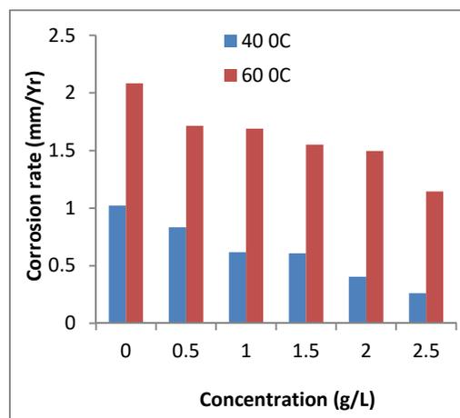
Fig.6: Corrosion rate of Pipeline steel in H<sub>2</sub>SO<sub>4</sub> with and without ECB at 40 and 60 °C
