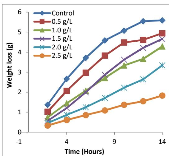
Fig.2: Variations in weight loss with time for pipeline steel coupons in 0.5 M H<sub>2</sub>SO<sub>4</sub> solution containing different concentrations of *Enantia chlorantha* at 40 °C
