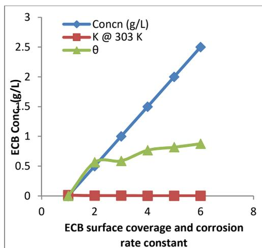
Fig.7: ECB concentration against ECB surface coverage and corrosion rate constant for pipeline steel corrosion in acidic environment at 30 °C (303 K)
