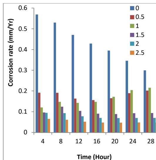
Fig.5: Corrosion rate of Pipeline steel in H<sub>2</sub>SO<sub>4</sub> with and without ECB extract at 30 °C
