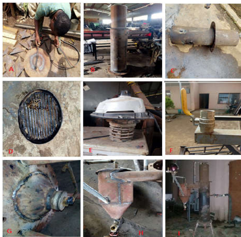
Where A = Cutting of flange plate; B = Flange welded with inner pipe; C = The outer and inner pipe forming the reactor; D = Attached air blower, E = Attached control valve, F = Fabricated grate; G = Fabricated ash collector, H = Fabricated filter I = Fabricated updraft gasify
