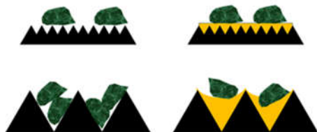
Fig 5. Illustration depicting both the dry (LHS) and oil-impregnated (RHS) of smaller (top) and bigger (bottom) particle-sized coatings. The smaller particle sized coating only allows the cells to rest on the tips of the textured coating and also provides a stable impregnated coated surface. The bigger particle-sized coatings possess large grooves that can accommodate cells and enhance stronger adhesion against turbulent flow and its impregnated coatings provides less stable oil surface.
