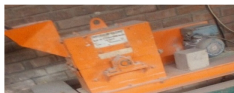
Fig 2: Broyeur-clero” hammer mill used for crushing
