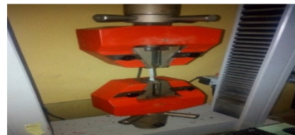
Fig 6: Testometric machine with the specimen wedged between its grips
