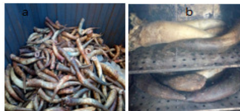
Fig 1: (a) Samples of the cow horns (b) The cow horn samples in the oven ready for drying
