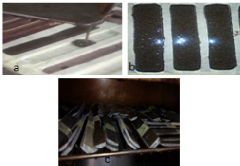
Fig 4: (a) Pouring of the cow horn mixture into the mould cavity, (b) Specimens at room temperature for curing, (c) Sets of specimens arranged in the oven for post curing
