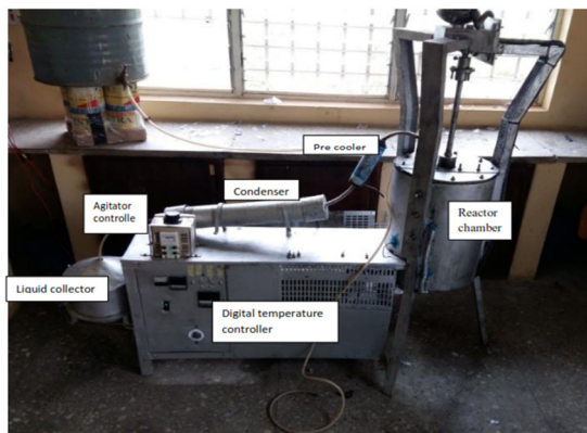
Plate 1: A laboratory scale pyrolysis rig
