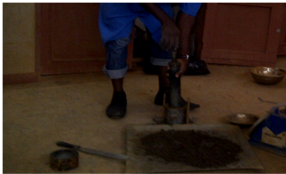
Plate 3: Compaction process for the lateritic soil-High Density Polyethylene waste mixture
