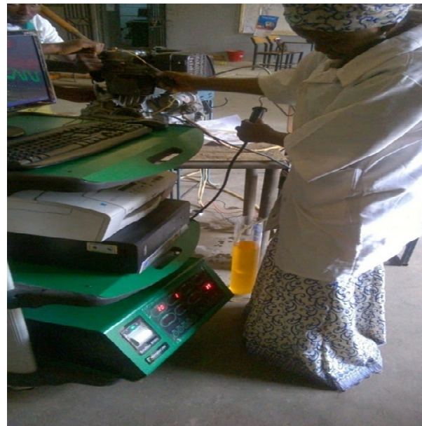
Plate I: Engine exhaust gas measurement (Motorscan 8050 gas analyzer).
