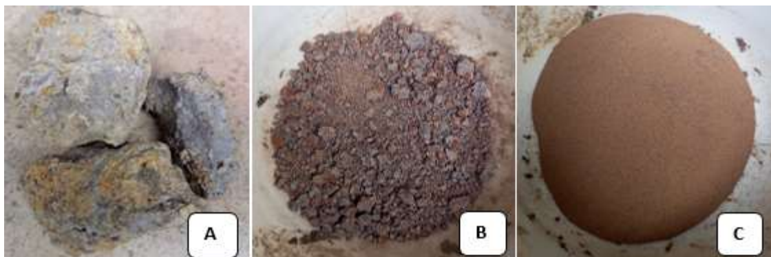
Fig 1 Clay sample preparation process. A) Raw clay sample. B) Crushed clay sample C) Sieved clay sample.
