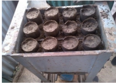
Fig 6: Moulding of briquettes
