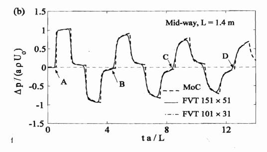
Figure 3: Pressure time history MoC solution and Finite-Volume Technique (FVT) solutions, computational mesh 151×51 and 101×31, for a 1.4 m long pipe (a) at the valve and (b) mid-way along the pipe
