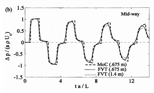
Figure 4: Pressure time history MoC solution, for a 0.675 m long pipe, and Finite-Volume Technique (FVT) solutions, for 0.675 m and 1.4 m long pipes,(a) at the valve and (b) mid-way along the pipe
