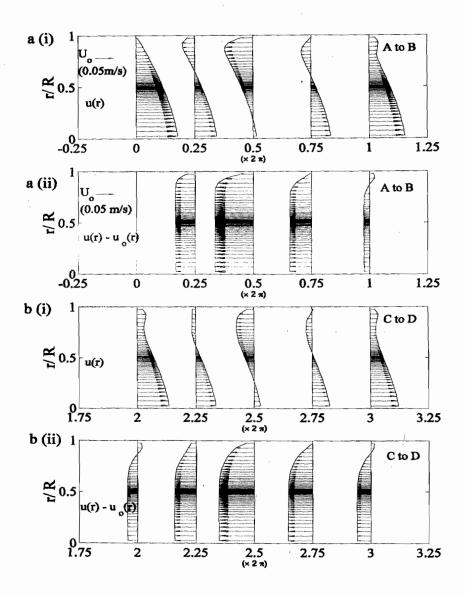
Figure 5: FVT velocity field solutions midway along the 1.4 m pipe shown as (i) overall velocity profile and (ii) velocity profile relative to initial steady state profile at different times in two cycle between (a) points A and B, and (b) points C and D shown in Figure 3
