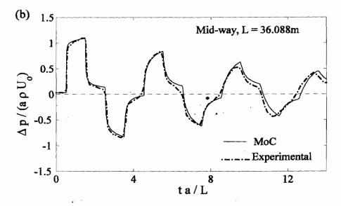
Figure 2: Experimental data and method of Characteristic (MoC) solutions for the pressure time history for a 36.088 m long pipe (a) at the we and (b) mid-way along the pipe
