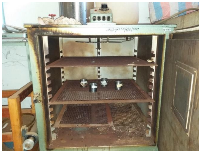
Fig. 1: Moisture determination using oven drying method
