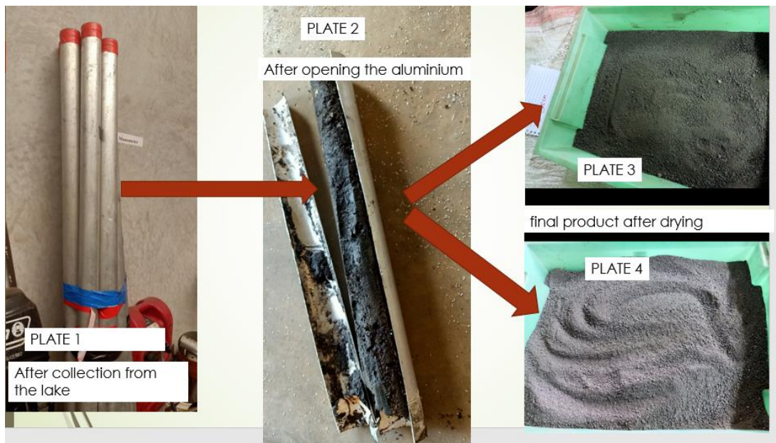
Figure 2: Drying, grinding, and sieving of the lake sediments in preparation for soil amendment.
