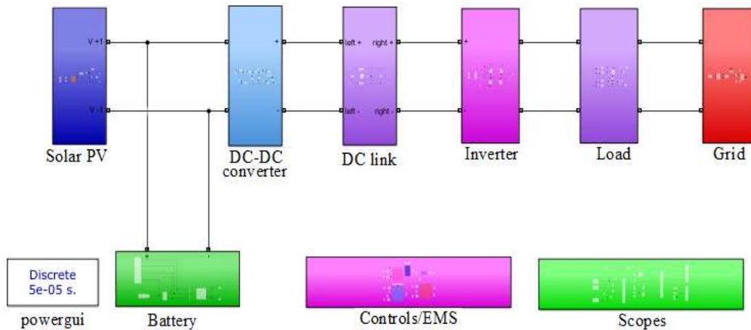
Figure 8. Simulink model of the Micro-grid system
