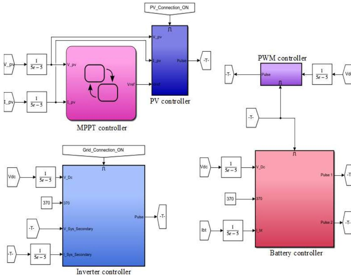
*Figure 9. Simulink model of energy management controls*
