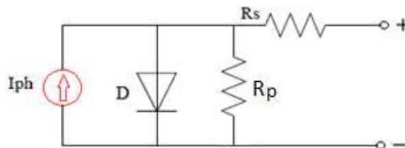
Figure 1. Single diode model with series and shunt resistors
