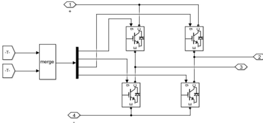
Figure 4. Simulink model of an Inverter
