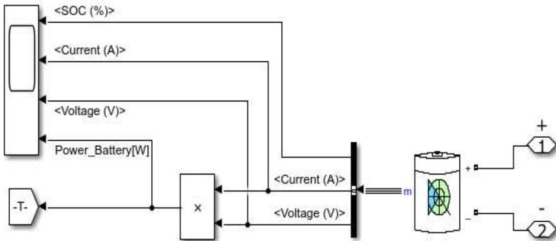
Figure 5. Simulink model of a Lead-Acid battery
