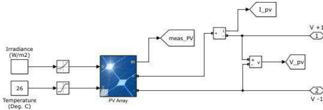
Figure 2. Simulink model of a solar PV
