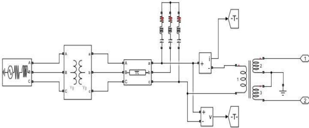
Figure 7. Simulink model of a power grid
