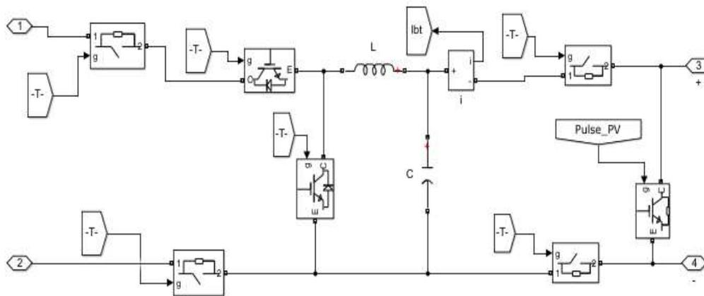
Figure 3. Simulink model of a DC-DC Converter
