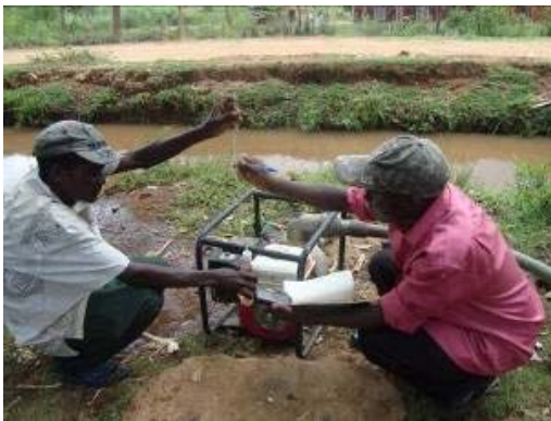
Photo 1: Measurement of fuel consumption rate of the pump
