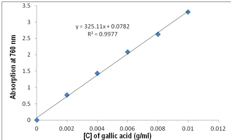
Figure 2: Calibration curve of Gallic acid
