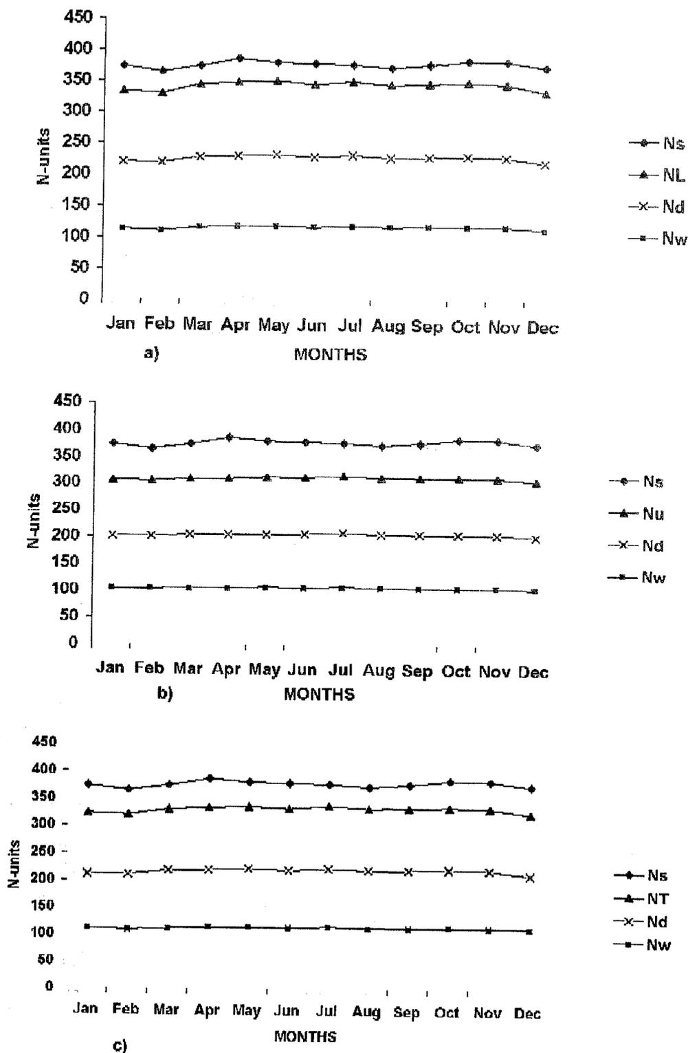
Fig. 1. Monthly variations of mean refractivity at different atmospheric levels and related parameters at Oshodi.
