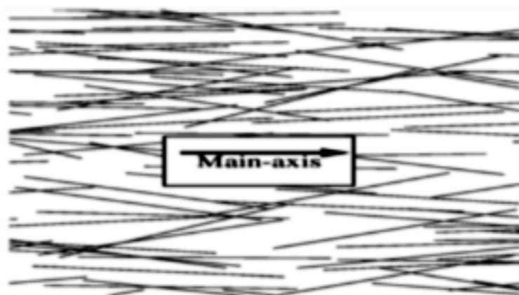
Figure 1. Illustration of fibers alignment in a substrate paper (Linder & Lofqvist, 2012).
