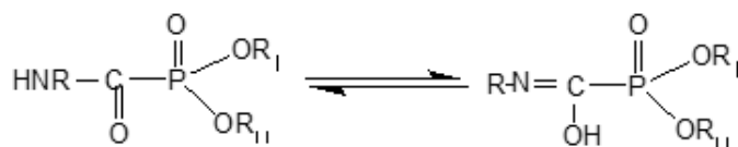
Figure 2: Typical keto-enol tautomerism in carbamoyl phosphonate.
