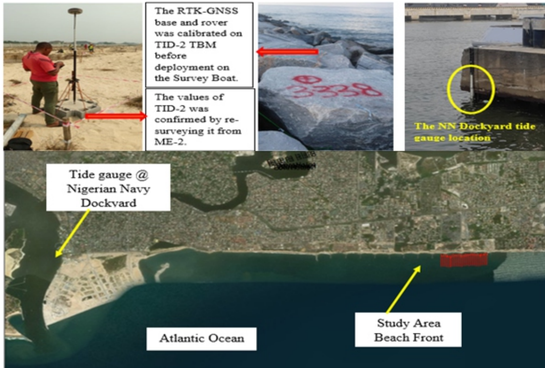
Plate 2: Locations of TID1 and TID 2 and the Nigerian Navy dockyard tide Gauge.
