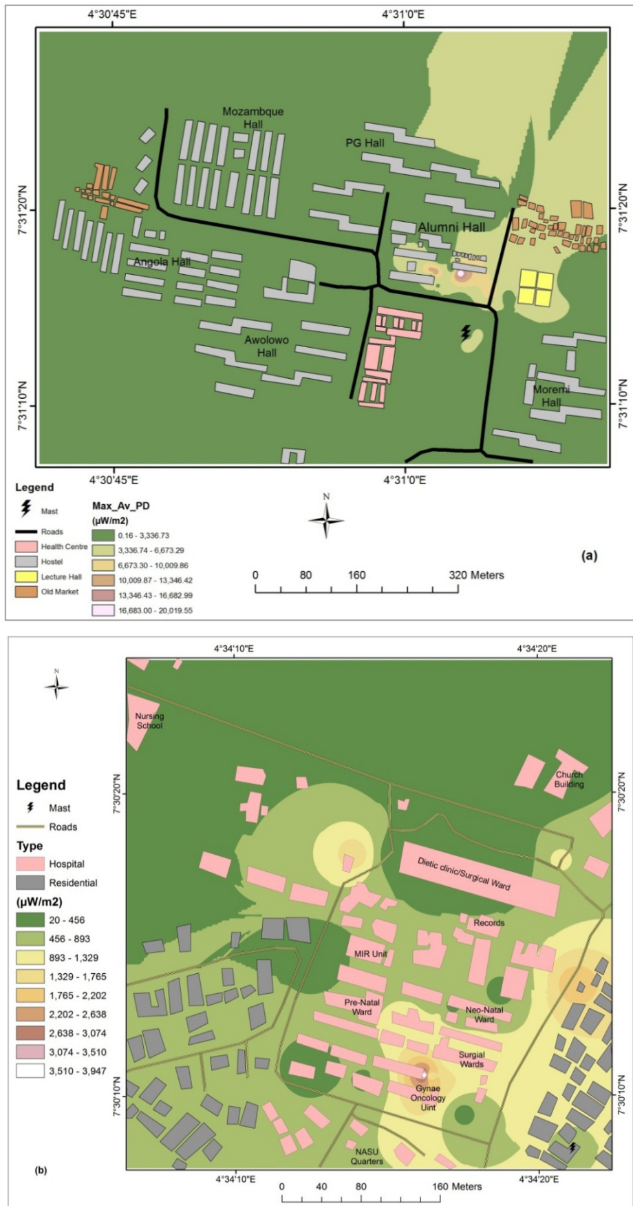
Fig. 5: Spatial Distribution of Maximum Average Power Density of Microwave Radiation at Students Hostel/Health Centre (a) and OAUTH Complex (b)
