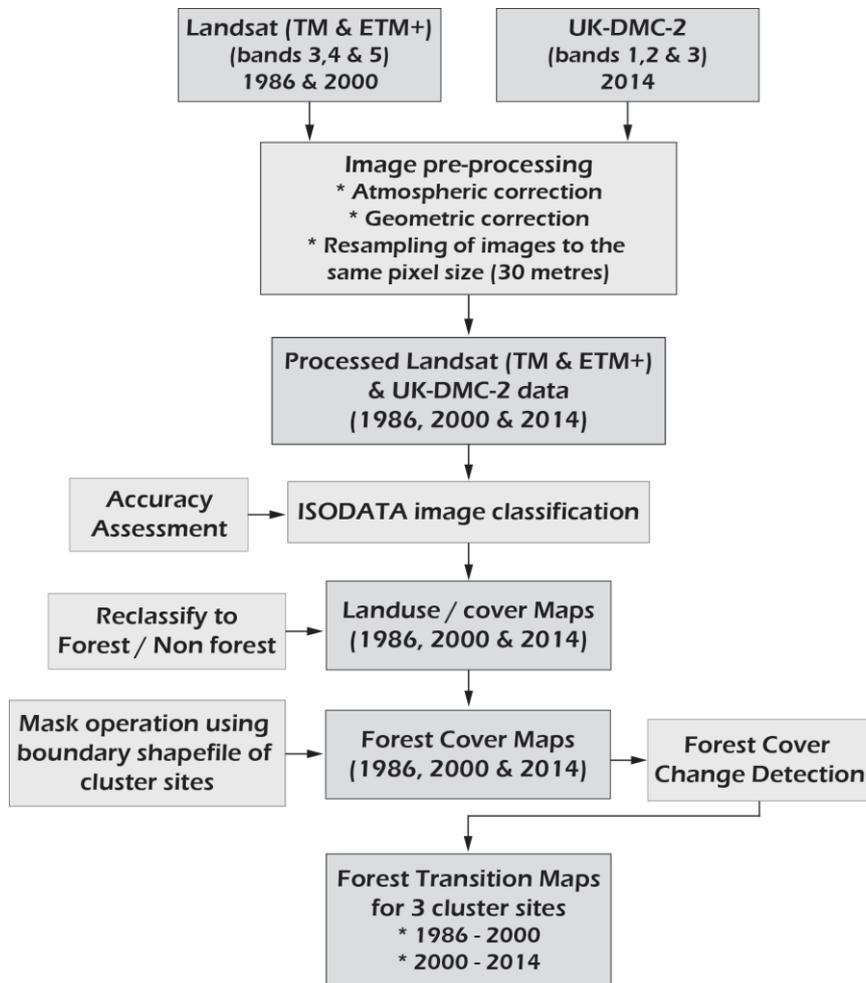
Figure 2: Workflow of Methodology Used for Image Processing
