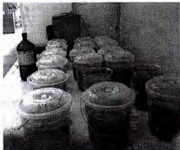
Plate 2: Soaking of concrete cubes in acid solutions using plastic bowls
