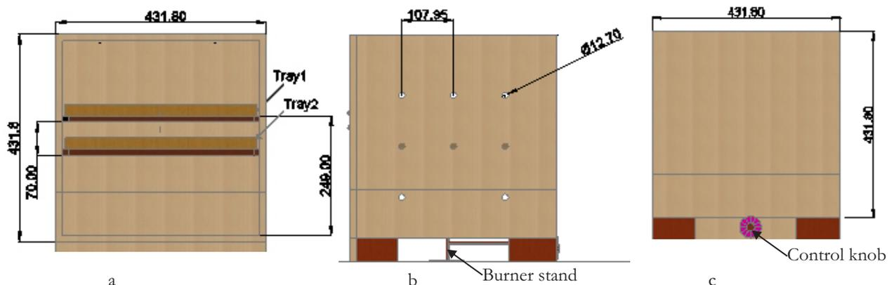
Figure 2 a- Schematic View of: a- Front, b- Side and c- Back walls of the Incubator (All dimensions in mm).
