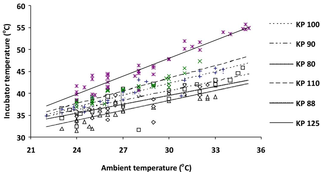
Figure 4 Calibration Curves of Chamber Temperature Against Ambient Temperature.
