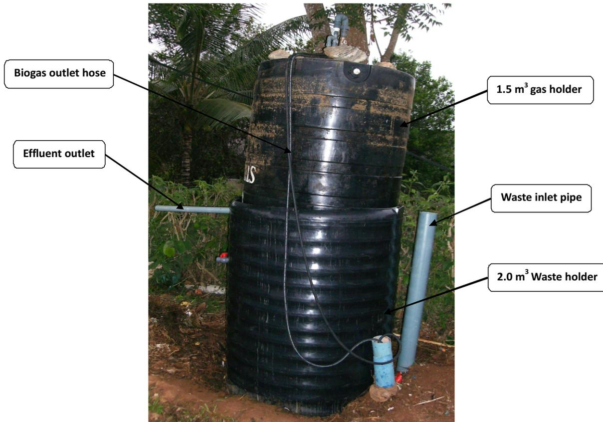
**Figure 3** Biodigester Used for Biogas Production.
