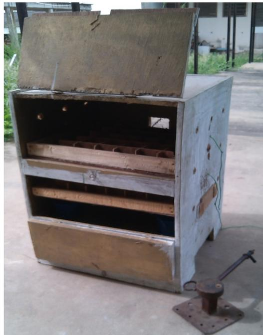
Figure 1 The Developed Incubator (with the Front Doors Opened) and the Biogas Burner.
