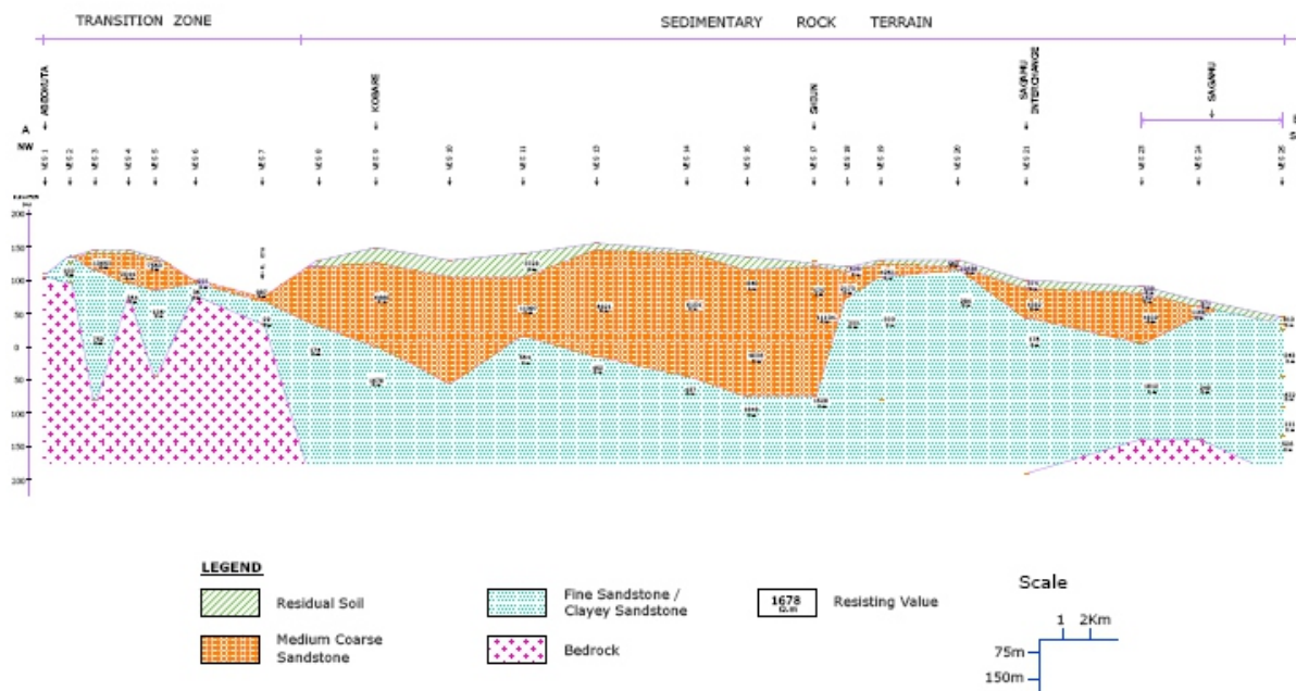
Fig 6 Geoelectric Section along Section A-B
