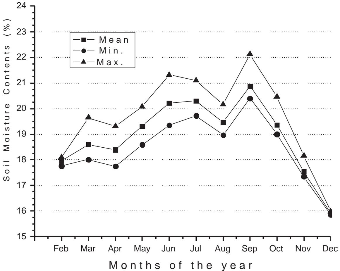
Figure 7: Monthly Variations for the Mean , Minimum and Maximum Values of Soil Moisture as Measured in 2006, in Ibadan
