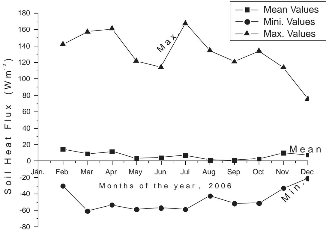
Fig.5: Monthly Variations for the Mean, Minimum and Maximum Values in Soil Heat Flux as Measured in 2006, at Ibadan.
