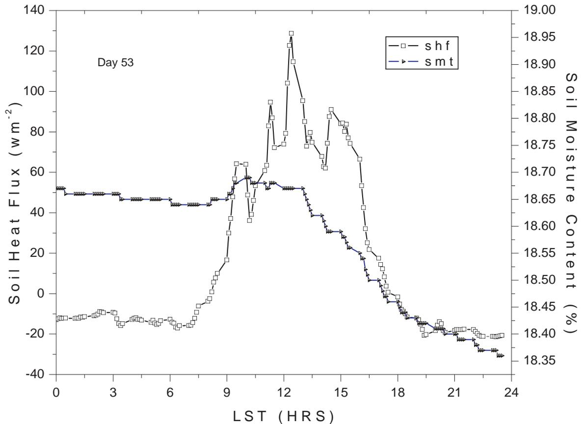
Fig. 2: Diurnal variation of Soil Heat Flux (s.h.f.) and Soil moisture Content (smt) of day 53, 2006 as Measured at the Nimex Site, Ibadan
