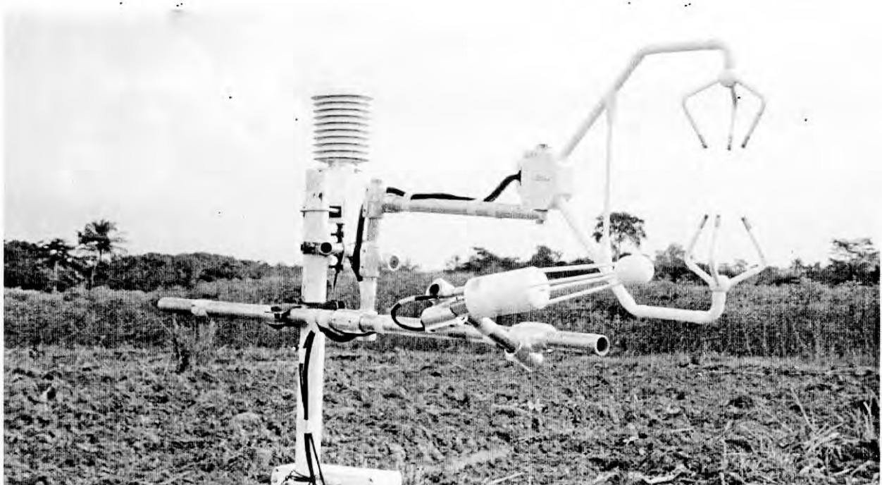
Figure 2: Photograph Showing Eddy Covariance System.
