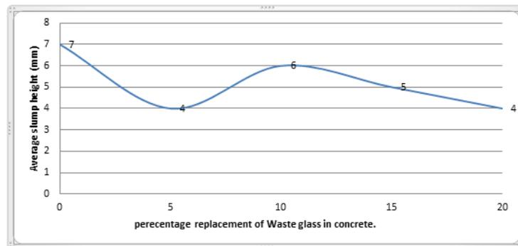
Fig 4: Average slump height against fine glass concrete
