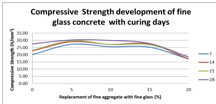
Figure 6: Graph of compressive strength development against curing days of modified concrete.
