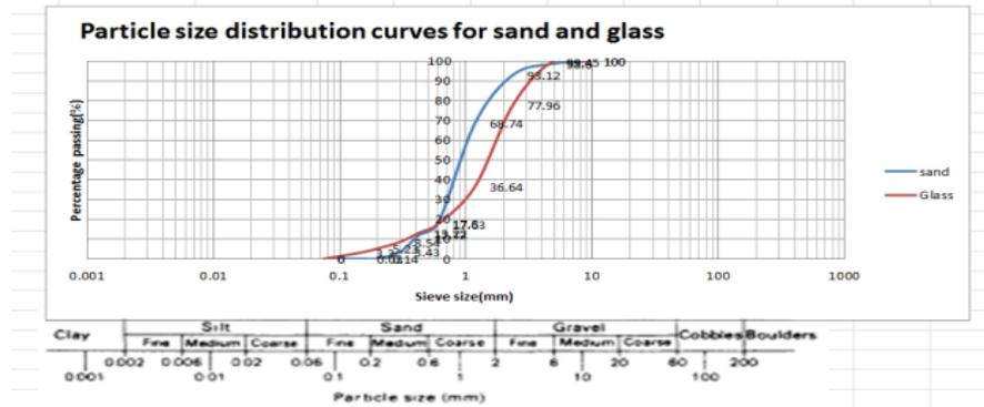
Fig .3: Particle size distribution for fine aggregate and crushed waste glass
