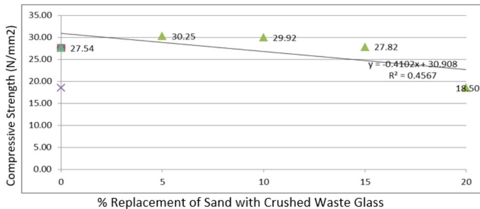
Figure 7: Compressive strength of waste glass concrete and percentage replacement of FWG in concrete.
