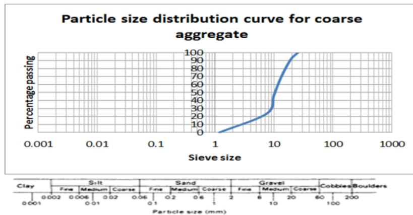
Figure 2: Particle size distribution curve for coarse aggregate (granite).
