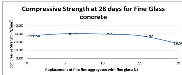
Fig 5: Graph of compressive strength at 28 days against percentage replacement of fine waste glass.
