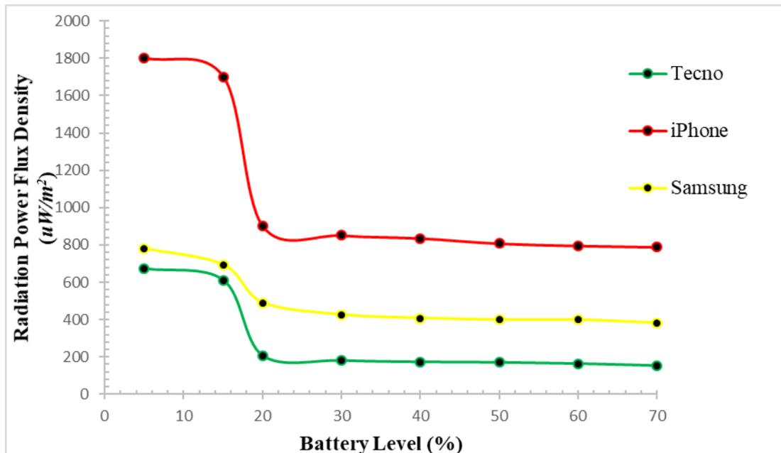
Figure 2: Radiation Level Profile as a Function of Battery Level
