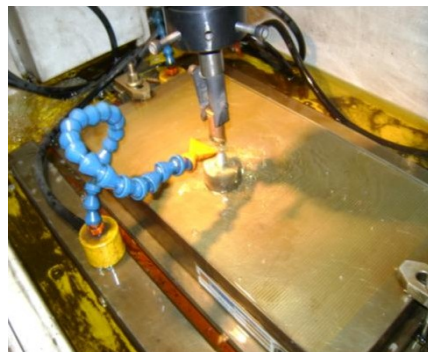
Figure 2: Jet flushing system
