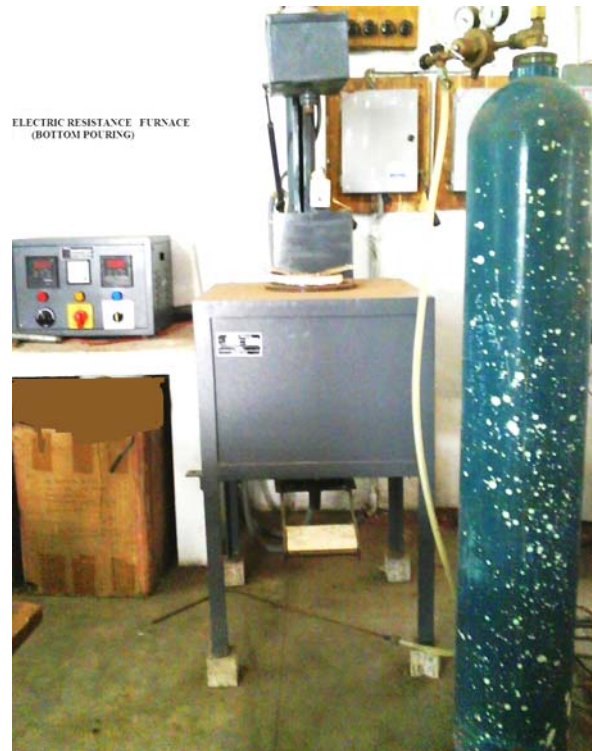
Figure 4: Experimental set up with bottom casting facility for synthesis of ALFA composites
