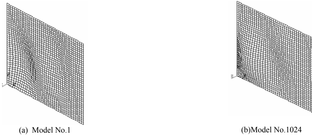
Figure 3. A pair of mirror image random imperfections plate models (amplitude enlarged by 50 times)
