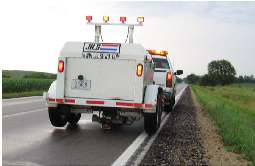
Figure 1. Non-destructive testing of pavements using Falling Weight Deflectometer (FWD)
