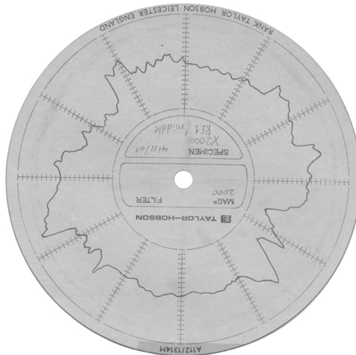
Figure 5. Roundness polar chart at 2000x illustrates circularity deviation created by turning with usual cutter at S = 0.07 mm/rev, t = 0.5 mm, and v = 3 m/sec.
